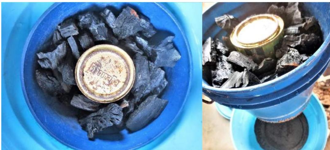
Self-constructed local refrigerator with the coffee lid-covered tin can in the centre surrounded by charcoal
